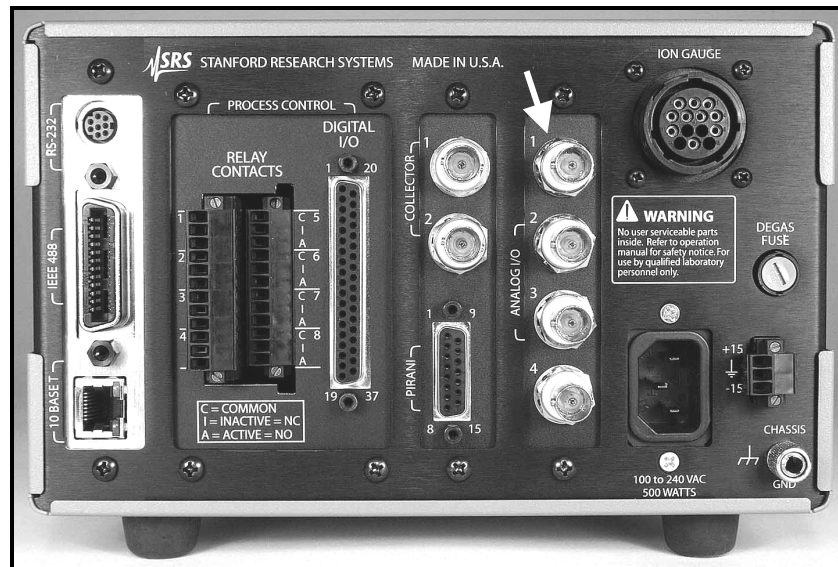
Figure 10-7. The four analog I/O ports.
