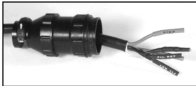
Figure 10-5. Gauge connectors of O100C3 cable.
