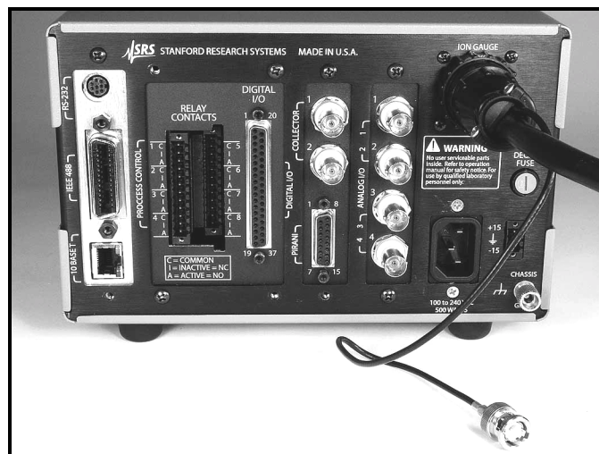
Figure 10-3. The 7-pin plug of the O100C3 cable is connected to the ION GAUGE receptacle on the back of the IGC100. The collector BNC is left unconnected.
