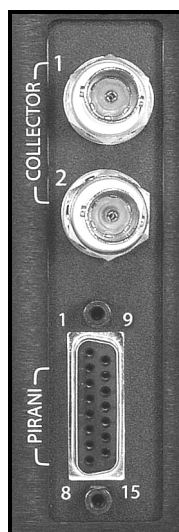
Figure 2-5. The Ion Gauge Collector BNC connectors.
