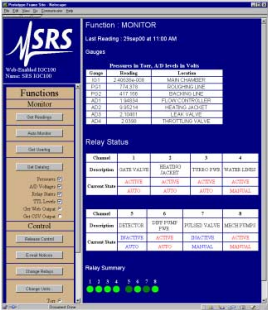
Figure 5-11. IGC100 web page showing relay status and control via the internet.
