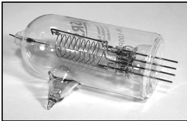
Figure 10-1. Sealed ionization gauge.
