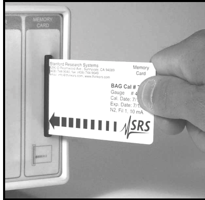
Figure 6-4. Insert the card into the controller.
