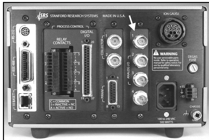
Figure 4-1. Rear panel Analog I/O ports.
